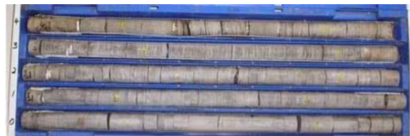
Weak Mudstone Core Obtained with a Lined TT56 Core Barrel
