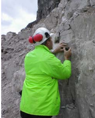
Orientation data collection using a CLAR compass
